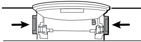
**Reassembly note** For ease of assembly, connect the IR wire assemblies to the optical sensors before attaching the handle cradle to the handle assembly housing.
